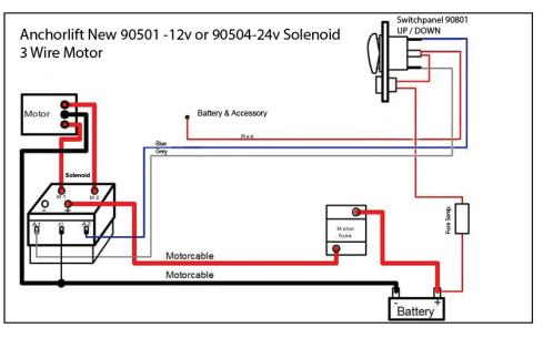
Wiring of ANY electrical item on a vessel should be done by a professional. We provide these wiring diagrams ONLY as a guide. If you are unsure or unable to properly install this item, we strongly recommend hiring a Marine Electrician.
