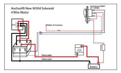
Wiring of ANY electrical item on a vessel should be done by a professional. We provide these wiring diagrams ONLY as a guide. If you are unsure or unable to properly install this item, we strongly recommend hiring a Marine Electrician.
