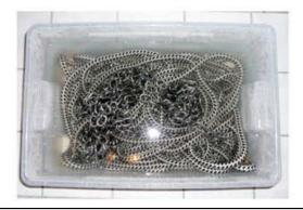
Fill a suitable container with fresh water. Ensure that all the rope is under water and soaked completely.
