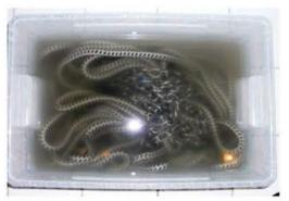
Move the rope around periodically so all the contaminants fall to the bottom of the container. (Move the rode around 3-4 times during a 1-2-hour period). Remove rode kit and place on a clean dry surface.
